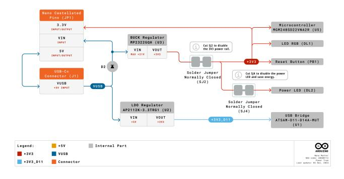
**Low-Power Tip:** For power efficiency, safely cut the LED jumper and connect an external +3.3 VDC power supply to the board's 3V3 pin. This configuration does not power the board's USB bridge.
