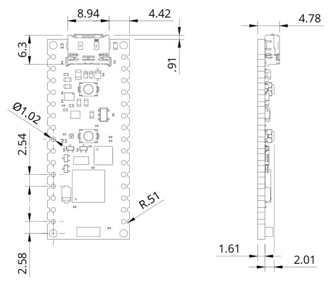
The Nano Matter was designed to be usable as a surface-mount module and presents a dual inline package (DIP) format with the Nano-styled header connectors on a 2.54 mm pitch grid with 1 mm holes.
